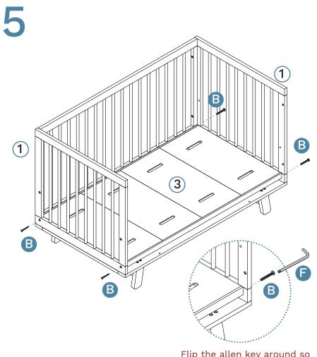
Flip the allen key around so the ball end is lined up with the screw/bolt.
